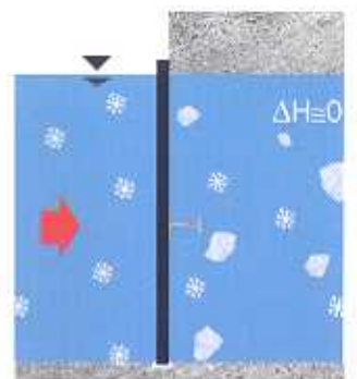
4. Ice breaks loose from thermoplastic blades. Hydrostatic pressure rapidly drops.
