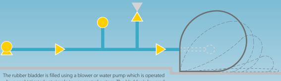
The rubber bladder is filled using a blower or water pump which is operated by a sophisticated yet simple to use control system. The bladder is lowered by means of an exhaust system, which is backed up by a mechanically operated failsafe deflation system in case of a power failure.
